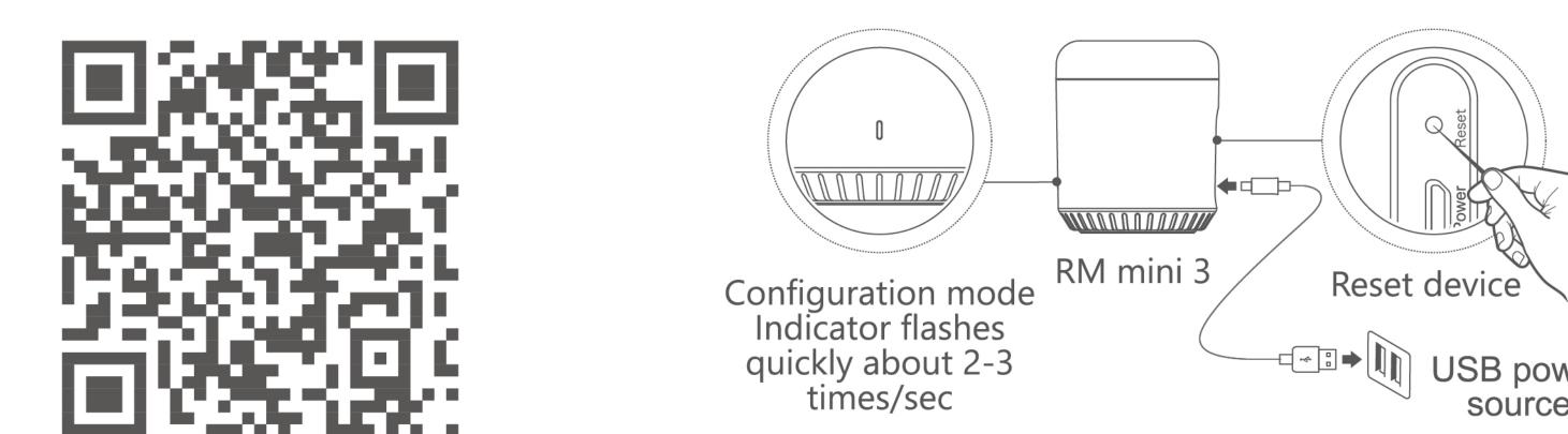
Power on the device with USB cable. If it is in first time use, the blue Wi-Fi LED will flash quickly (about 2-3 times per second) indicating the device is in configuration mode (waiting to be added into
